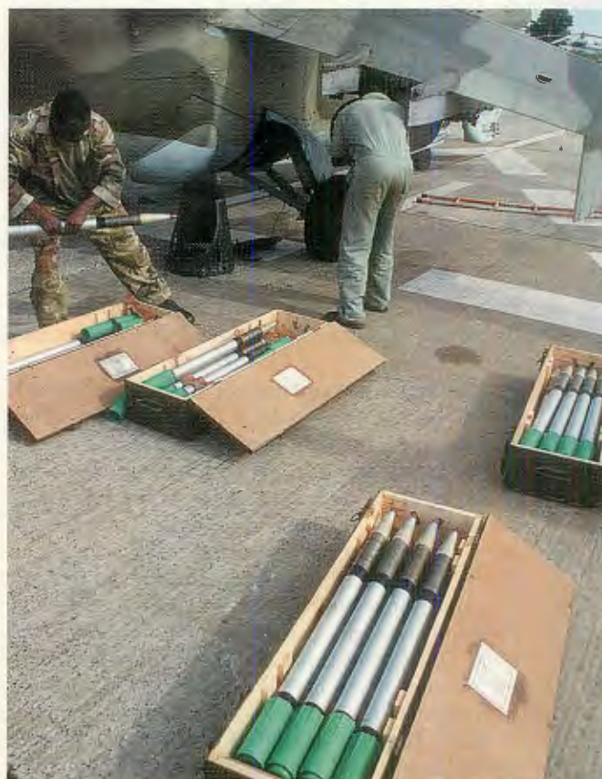
Hind gunship is prepared for a sortie in Sierra Leone with 80mm air-to-ground rockets. Unlike with the more common NATO 57mm rockets, gunships have to stand off a bit when using the larger projectiles to avoid their own shrapnel salvos.
