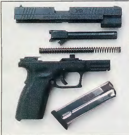
Here the XD-40 Tactical is seen field-stripped. The pistol comes apart without the need for tools and goes back together in seconds.
